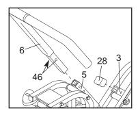
(46) and slide the Handlebar Assembly (6) out of the Handlebar Swing Arm (5). Press the Snap Buttons again and insert the Handlebar Assembly into the Wheel Swing Arm (3). **Make sure that the Snap Buttons snap into the holes in the Wheel Swing Arm.** Press the Swing Arm Cap (28) onto the Handlebar Swing Arm (5).
